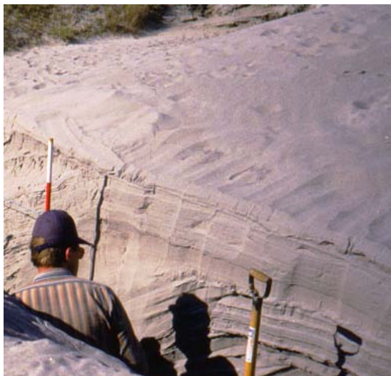
Figure 2-10. Heterogeneity in apparently homogeneous materials. Exposure of a sand dune, showing its heterogeneous, anisotropic structure. (Photo courtesy University of Chicago.)
